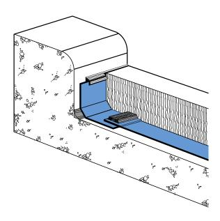
The membrane is highly resistant to water and deicing salt solutions. Electrical resistance measurements on structures have been exceptionally high to indicate the effectiveness of Bituthene 5000 in preventing water migration into decks.
